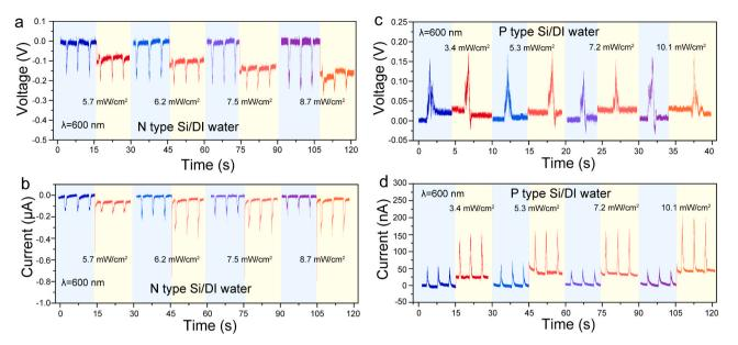
Fig. 3. Effect of light intensity on the coupling interaction between photovoltaic effect and tribovoltaic effect. The effect of light intensity on the (a) tribo-voltage, (b) tribo-current between the DI water and the N-type Si. The effect of light intensity on the (c) tribo-voltage, (d) tribo-current between the DI water and the P-type Si.
