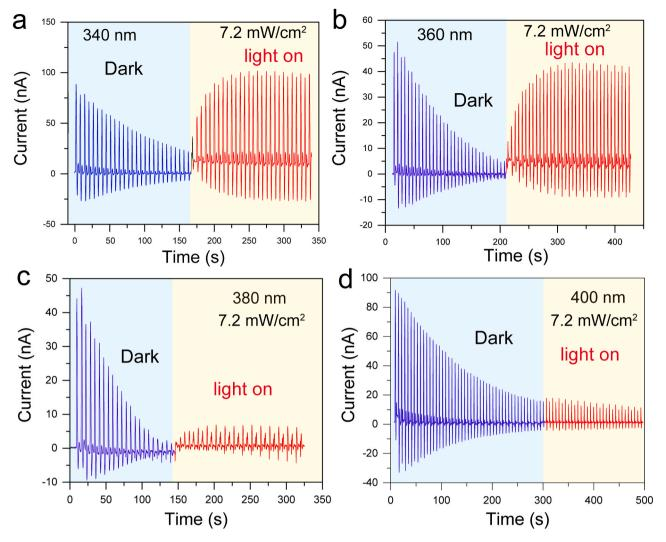
**Fig. 4.** The coupling of photovoltaic effect and tribovoltaic effect at the DI water and the  $TiO_2$  interface. The oscillogram of the short-circuit current when a DI water droplet slides on a  $TiO_2$  surface in the dark condition and under light irradiation with (a) 340 nm, (b) 360 nm, (c) 380 nm, (d) 400 nm light wavelengh, 7.2 mW/cm<sup>2</sup> light intensity.
