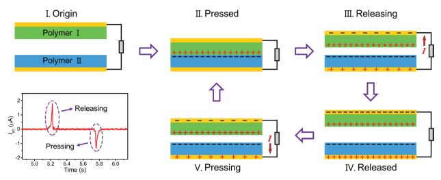
Figure 2. Sketches illustrating the working principle of the TENG in contact-separation mode.
