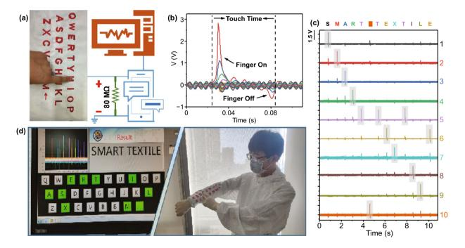
**Fig. 5** Working principle of the self-powered wearable keyboard as a biometric self-recognition system. **a** Schematic diagram of a SPWK working with a terminal device. **b** A diagram of a voltage signal when a finger strikes a single keypad. **c** Signal output waveform by continuously typing the string of "SMART TEXTILE" that is recorded in real time without uncomfortable delay. **d** Photograph showing the SPWK system for the real-time keystroke tracing and recording
