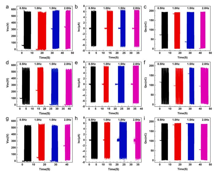
Fig. 3. Performance of the CO-TENG for harvesting random mechanical energy. (a-c) Electric output characteristic at different frequencies with a fixed amplitude of 20 mm; (d-f) electric output characteristic at different frequencies with a fixed amplitude of 35 mm; (g-i) electric output characteristic at different frequencies with a fixed amplitude of 50 mm; (a), (d), (g) open-circuit voltage; (b), (e), (h) short-circuit current; (c), (f), (i) transfer charge.
