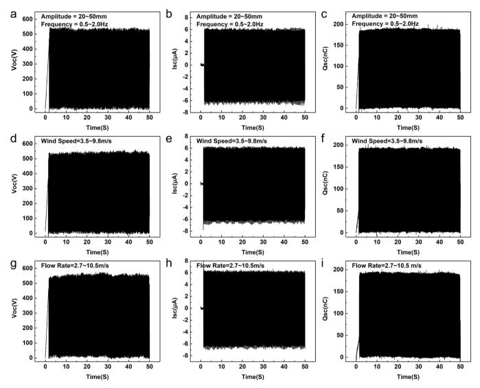
Fig. 4. Demonstration the electrical output characteristic of the CO-TENG for harvesting ambient natural environments. (a-c) Electrical output characteristic under random wave energy; (d-f) electrical output characteristic under random wind energy; (g-i) electrical output characteristic under random water energy.
