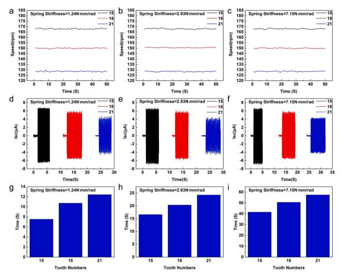
Fig. 2. Rotor speed, running time, and short-circuit current of the CO-TENG under fixed excitation conditions. Top row: Rotor speed under different numbers of ratchet teeth and same spiral spring stiffness; Middle row: Short-circuit current response to different numbers of ratchet teeth and same spiral spring stiffness; Bottom row: Running time on different numbers of ratchet teeth and same spiral spring stiffness.
