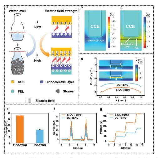
Figure 2. The schematic mechanism of field enhancing breakdown effect. a) Schematic mechanism of field enhancing breakdown effect by adding FEL. b–d) Electric field distribution and the electric potential simulation between charge collection electrode and electrification in conventional DC-TENG and E-DC-TENG. e) Transferred charge in a cycle, and f)  $I_{sc}$  and g)  $V_{oc}$  outputs of conventional DC-TENG (blue line) and E-DC-TENG (yellow line).
