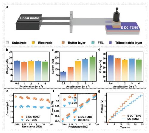
**Figure 3.** Output performance of sliding mode E-DC-TENG. a) Representative diagram of sliding mode E-DC-TENG. b) Transfer charge and c) peak of  $l_{sc}$  and d)  $V_{oc}$  outputs of E-DC-TENG at different accelerations. e) Instantaneous peak current and f) power of conventional DC-TENG and E-DC-TENG with various resistances. Inset shows the magnification of power. g) Measured voltage of a capacitor (30 nF) charged by a sliding mode E-DC-TENG.
