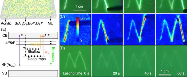
**FIGURE 2** Visual sen-memory of the pressure. (A) Schematic of the device in conjunction of ML hybrids and phosphor embedded in acrylic matrix for the visual sen-memory of the pressure. (B,C) The photographs and the corresponding intensity maps of the device during the sen-memory process of the applied force. (D) The afterglow images of the device after the removal of the applied force. (E) Schematic illustration of the sen-memory mechanism
