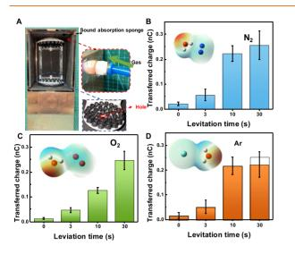
Figure 4. Contact electrification between levitated water droplets and different kinds of gases. (A) Photograph of sealed acoustic levitation equipment with two ultrasonic emitter arrays. A hole is in the middle of the bottom array in order to let the water drop into the Faraday cup. The transferred charge (from Faraday cup) of the DI water droplet with different levitation time (B) in a N<sub>2</sub> atmosphere, (C) in an O<sub>2</sub> atmosphere, and (D) in an Ar atmosphere.
