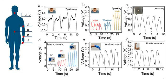
Figure 4. Demonstration of the self-powered sensor for detecting subtle mechanical motions. The sensor is attached to the throat for (a) swallowing and (b) speaking detection; and (c) breathing detection by attaching it on the belly. (d,e) Signals of human joint motion from the fingers and wrist. (f) Voltage of the sensor induced by the muscle movement.
